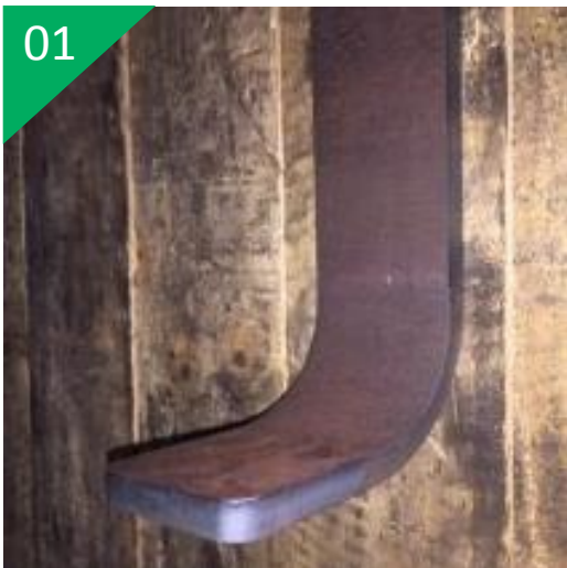
WEL-TEN590RE in 12mm thickness after bending process.
